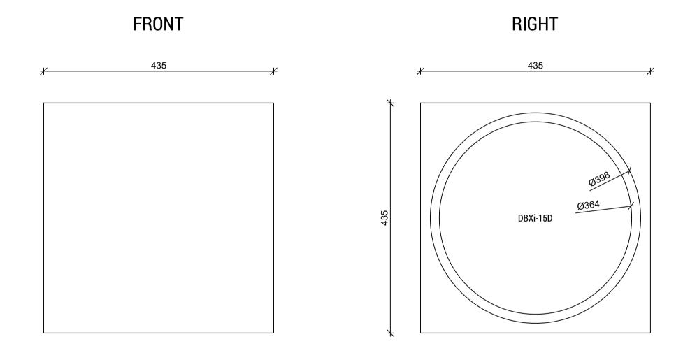
Earthquake Supernova MKVI-15 Front and right faces, scale 1:5, paper size A4 (ISO 216), revision 1.0 Measurements are in mm - these drawings are provided as-is, and all use of these are under your own responsibility.
